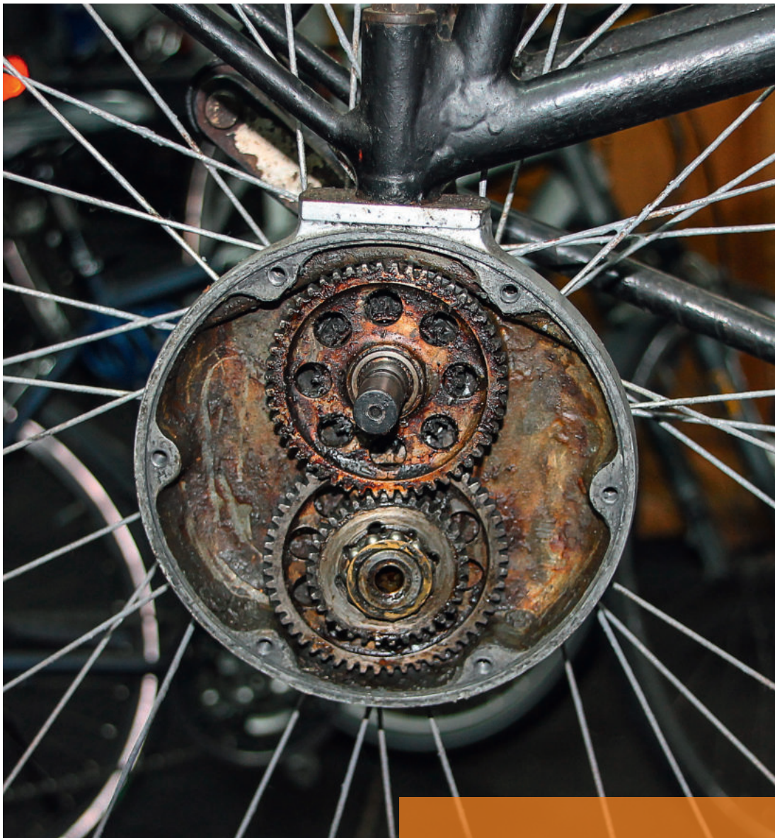
↑ The gears of a genuine Woerner bike: Exact dimensions for the design drawings formed the basis of the award-winning apprentice project.
